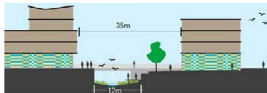
Daylighted water course
