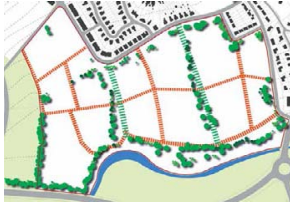
Street structuring for gravity surface drainage
