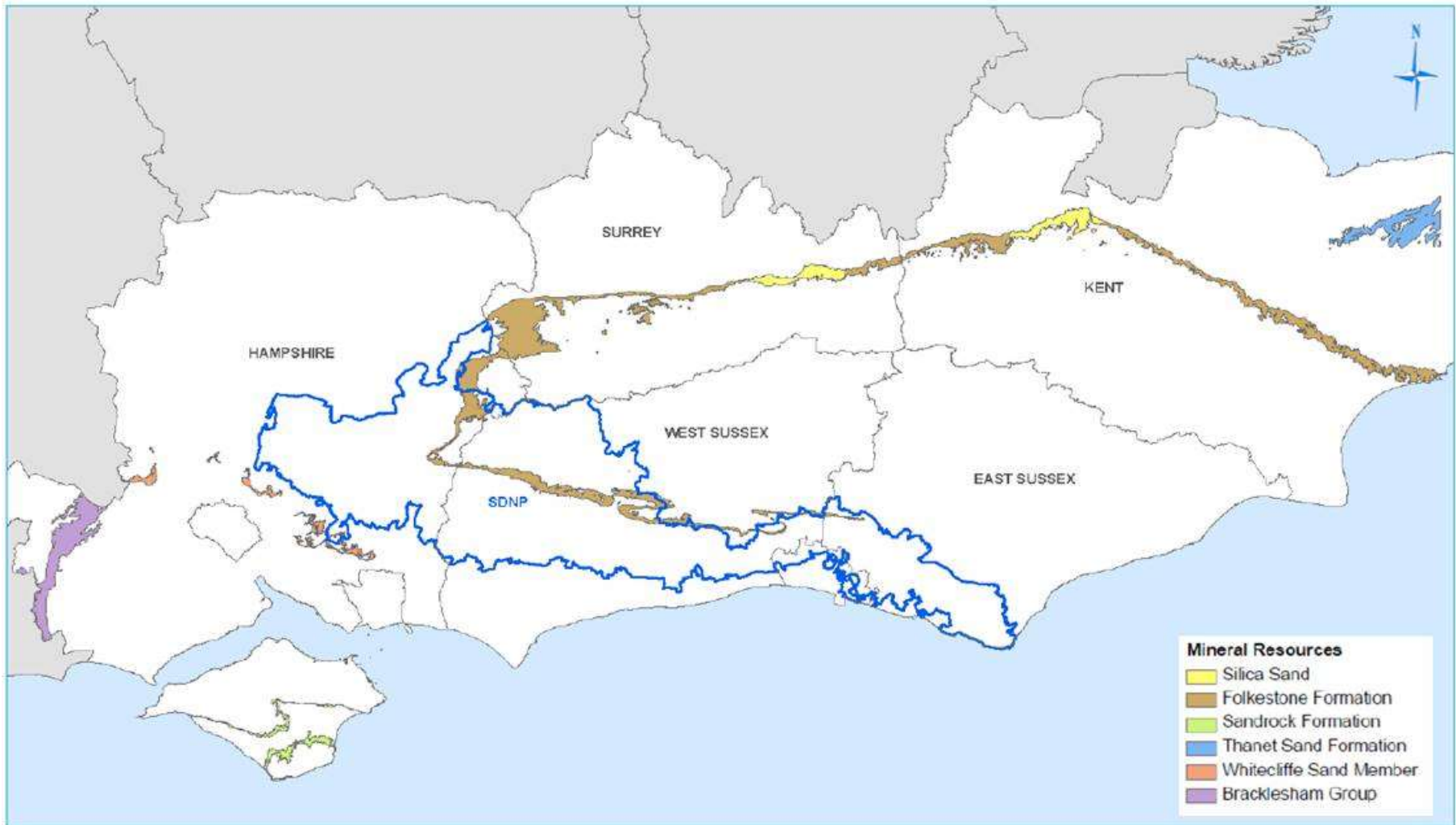
Figure 2: The Folkestone Formation and other soft sand resources in South East England.
