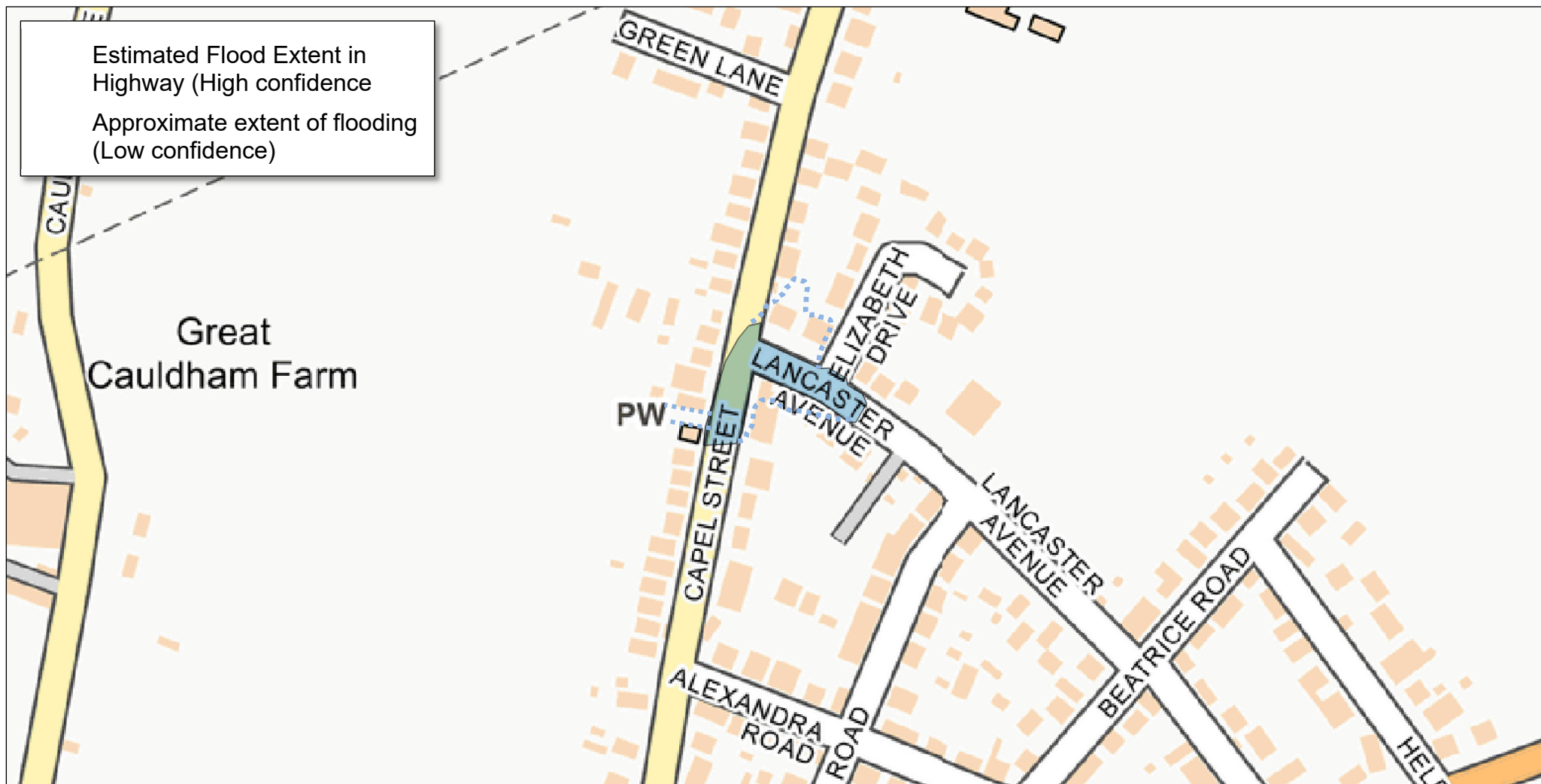
Annex 1 – Estimated flood extent of reported flood incident in Capel-le-Ferne. The estimated flood extent covers the roads only and not the properties which experienced flooding.
